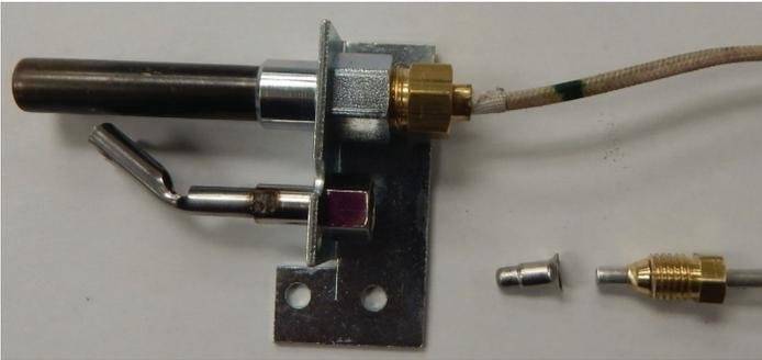
6. Remove the main burner orifice and replace with Propane main burner orifice supplied in conversion kit. The orifices included in this kit are stamped with their sizes. Use the correct orifice for your burner, as called out in the parts list table. Using the wrong orifice will result in improper burner operations. Set Air Shutter to full open before reinstalling Brass Elbow.
