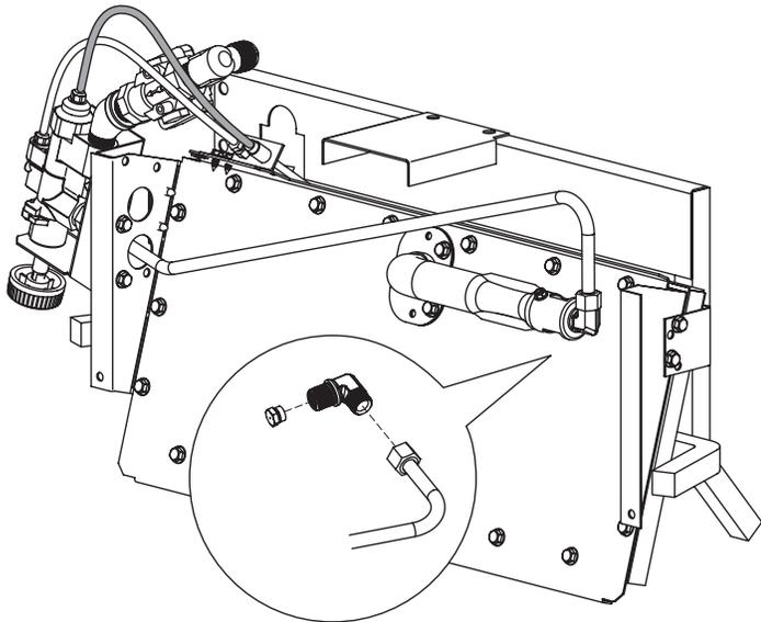
7. Remove inline regulator marked 5.3 on gas valve assembly.
