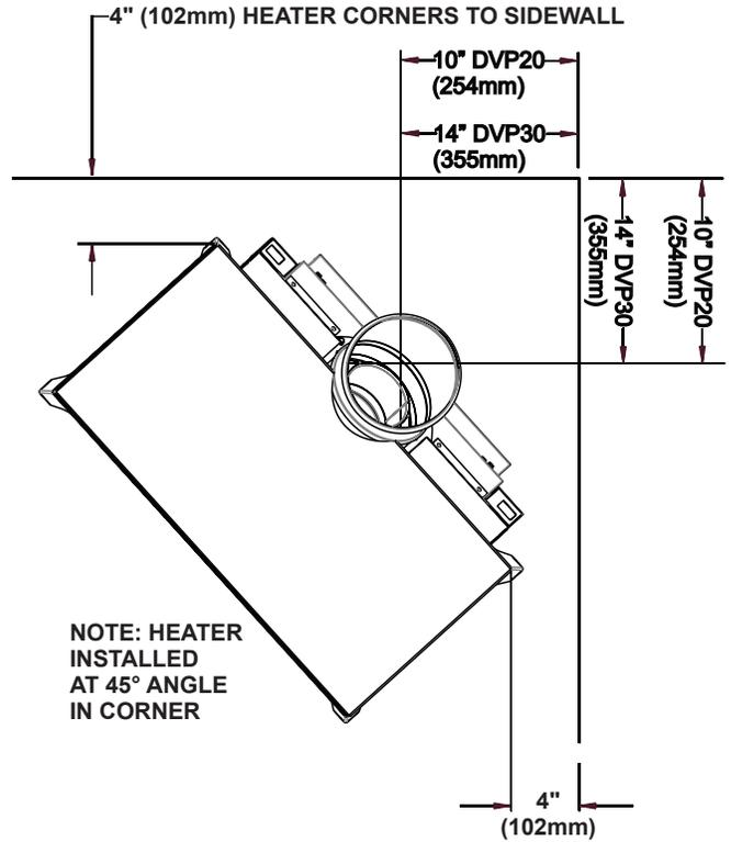
NOTE: HEATER INSTALLED AT 45° ANGLE IN CORNER
