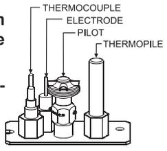
9. Push in gas control knob all the way and hold in. Repeatedly push the Piezo Ignitor Button until the pilot is lit. Continue to hold the control knob in for about one minute after the pilot is lit. Release knob, and it will pop back up. Pilot should remain lit. If it goes out, repeat steps 5 through 9.
