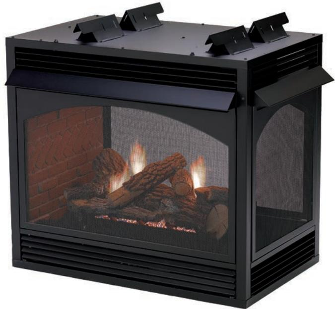
*The Vail Premium 36-inch Peninsula Vent-Free Fireplace includes a 38,000 Btu Slope Glaze Vista Burner, plus fixed screens, louvers, and hoods on three sides. Requires Rock Creek refractory log set. Also available in See-Through model with two open sides*
