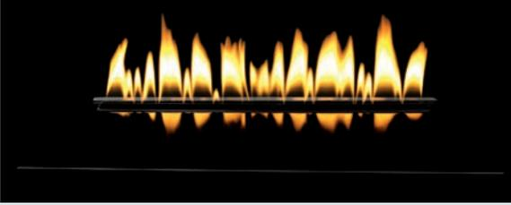
Empire also offers three styles of decorative glass to conceal the burner and create the illusion of flame floating above a reflective field. All of the glass starts as tempered panes that are shattered, screened for the proper particle size, and tumbled to minimize sharp edges.
