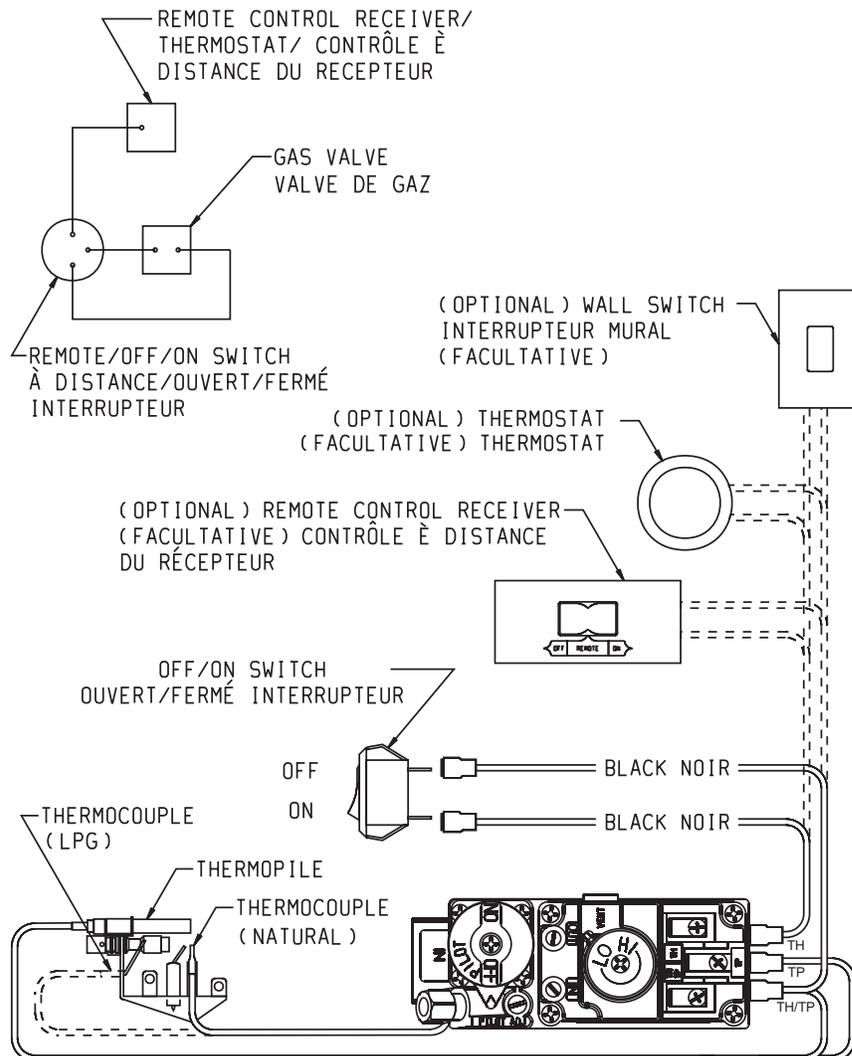
IF ANY OF THE ORIGINAL WIRE AS SUPPLIED WITH THIS UNIT MUST BE REPLACED, IT MUST BE REPLACED WITH NO. 18, 150°C WIRE OR ITS EQUIVALENT.
