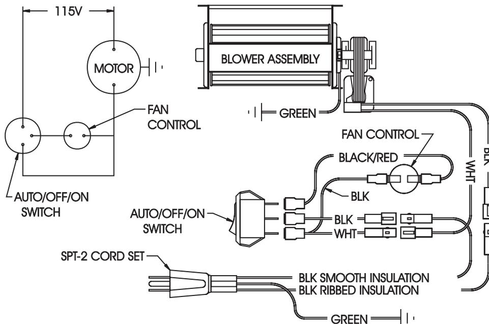
IF ANY OF THE ORIGINAL WIRE AS SUPPLIED WITH THIS UNIT MUST BE REPLACED, IT MUST BE REPLACED WITH NO. 18 GAGE 150°C 2/64 INSULATION WIRE OR ITS EQUIVALENT.
