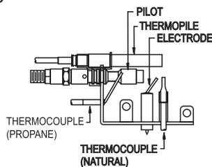
9. Push in control knob all the way and hold in. Repeatedly push the Piezo Ignitor Button until the pilot is lit. Continue to hold the control knob in for about one minute after the pilot is lit. Release knob, and it will pop back up. Pilot should remain lit. If it goes out, repeat steps 5 through 9.
