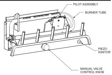
Thermostat Valve for VFDT Series Figure 16
