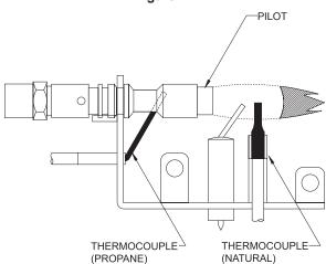
Incorrect Flame Pattern for VFDT & VFDM Figure 22
