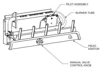
Manual Valve for VFDM Series Figure 17
