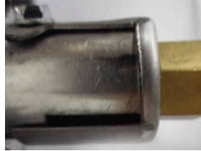
**Figure 1 - Air shutter at 1/8-inch opening**
