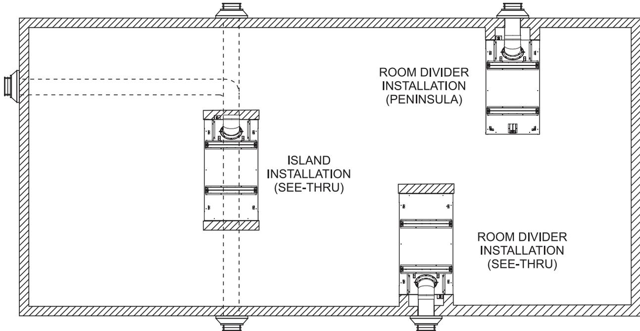
**NOTICE:** Island and Room Divider installation is possible as long as the horizontal portion of the vent system does not exceed 20 feet with a minimum vertical run of 8 feet from fireplace floor. See details in Venting Section.
