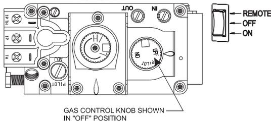
**NOTICE:** Knob cannot be turned from "PILOT" to "OFF" unless knob is pushed in slightly. Do not force.
