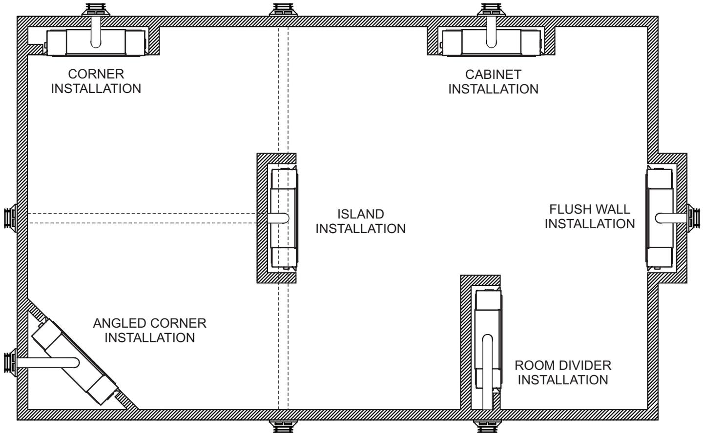
Note: Island and Room Divider installation is possible as long as the horizontal portion of the vent system does not exceed 20 feet with a minimum vertical run of 8 feet. See details in Venting Section.
