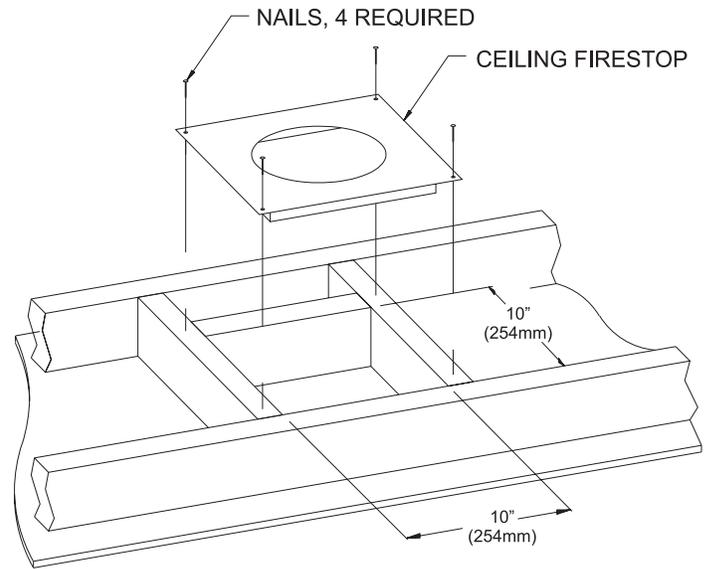
**Figure 50 (Attic Installation)**
