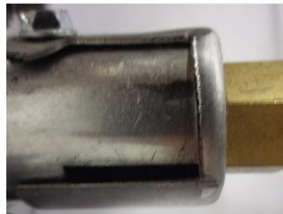
**Figure 6 (1/16-inch opening for natural gas models)**
