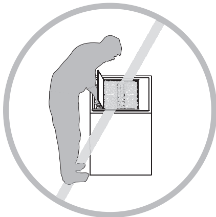
NEVER LEAN OVER FIREPIT WHEN LIGHTING BURNER
