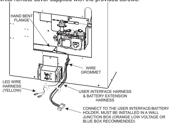
**NOTICE:** OUTER ACCESS DOOR REMOVED. REPLACE AFTER ALL WIRE AND GAS CONNECTIONS HAVE BEEN MADE.
