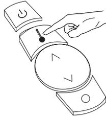
2. When the remote is activated, the fireplace display panel will illuminate and show Flame Level 1 along with the remote signal symbol. The fireplace will begin the start up sequence automatically.
