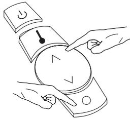
4. Once the desired program is selected, press the menu button to save the setting and return to the remote's home screen. The outline of the clock icon indicates that the program mode is active.
