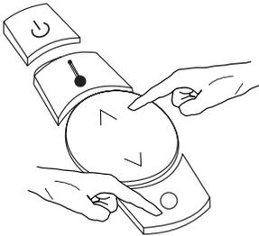
4. If the remote has the batteries installed but the time and date need to be adjusted, turn off the remote by holding down the power button until the display back light turns off.
