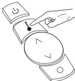
2. When the remote is activated, the fireplace display panel will illuminate and show the flame level set by the remote along with the remote signal symbol. The fireplace will begin the start up sequence automatically
